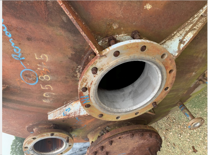
SS Nozzle with carbon steel support gussets
