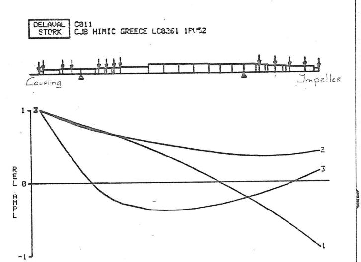
The undamped critical speed mode shapes are plotted based upon oil film stiffness at  $290 \circ R.P.M.$
