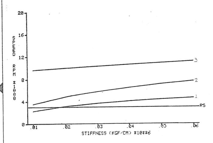
Lateral critical speeds are plotted against support stiffness. The effect of damping is neglected.
