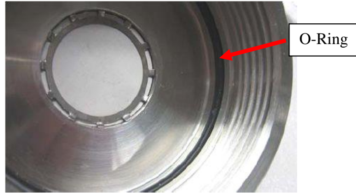
Figure 46 - Installed Retainer Ring
