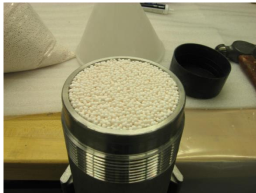
Figure 51 - Topped off Desiccant
