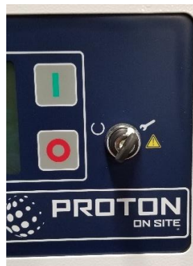
Figure 9 - Key in Service Bypass Mode
