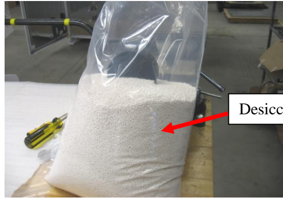
Figure 49 - Filling Dryer Cylinder and Desiccant
