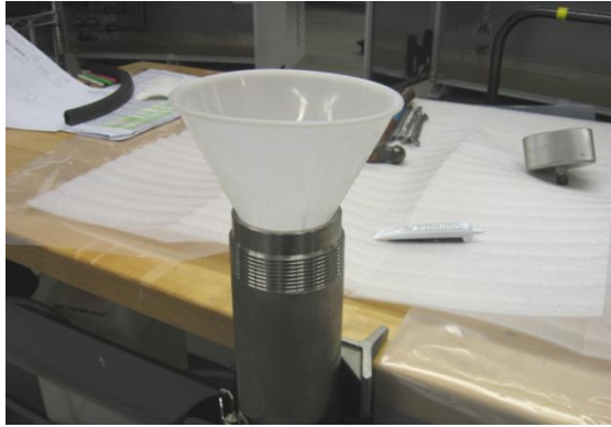
Figure 49 - Filling Dryer Cylinder and Desiccant
