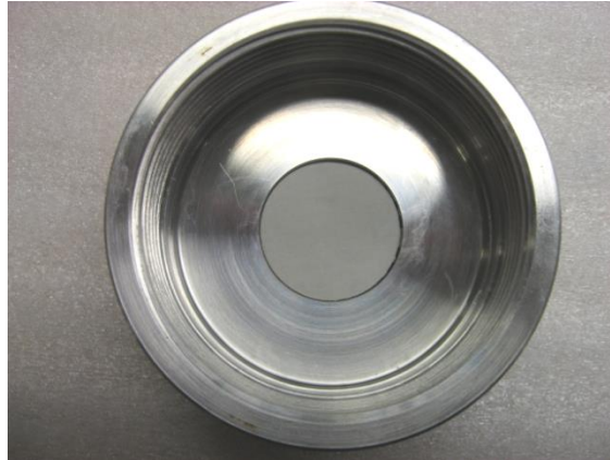
Figure 44 – Cap with Filter Screen
