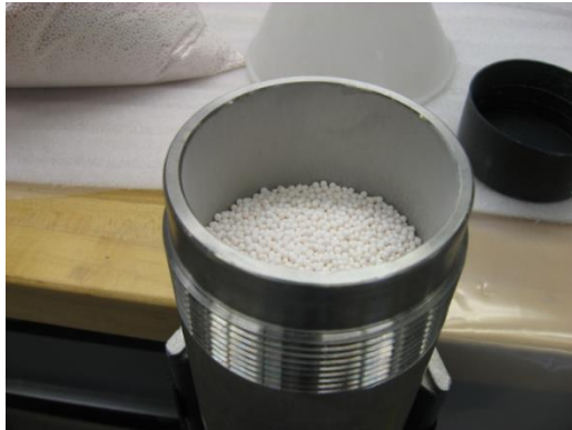
Figure 50 - Desiccant at the Top of the Cylinder and Tapping the Cylinder
