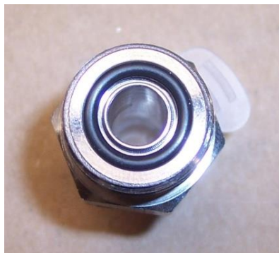
Figure 48 - Dryer Fitting with O-Ring
