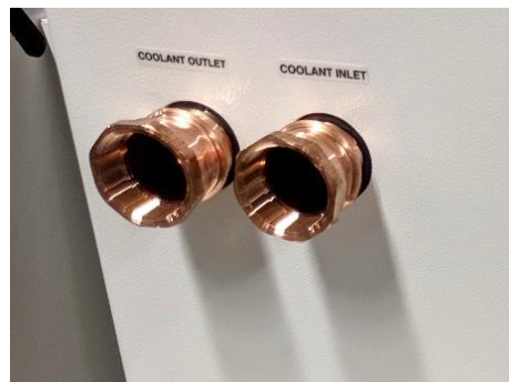
Figure 24 - Power Supply Enclosure Coolant Interfaces
