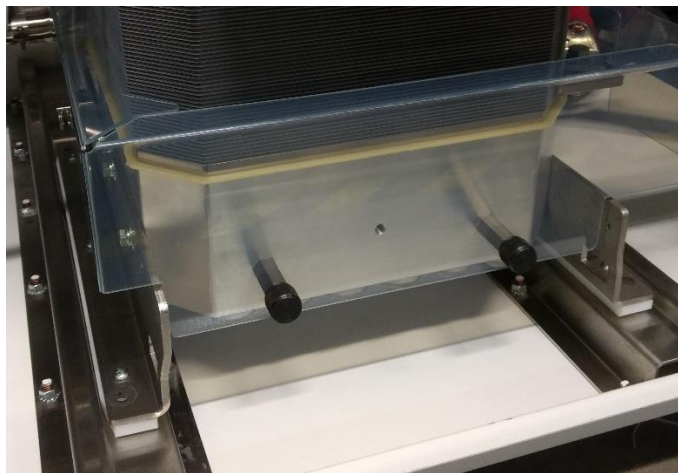
Figure 51 - Positive bus terminal cover
