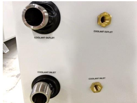
Figure 23 - Electrolyzer Enclosure Coolant Interfaces
