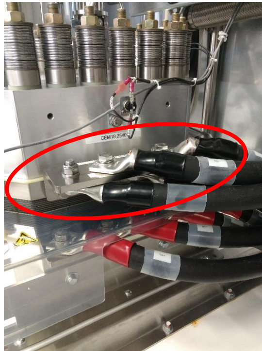
Figure 52 - Cell Stack Return (DC-) Terminal Connection
