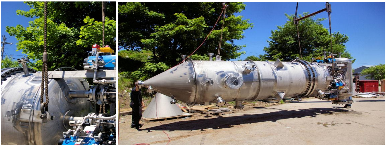
Figure No. 6.1: Mott GSV Filter Top Head Lifting Lugs & Shell Tailing Lug
