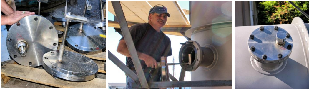
Figure No. 5.3: Mott GSV Filter Vessel Special Shipping Support Fixtures (Typical)
