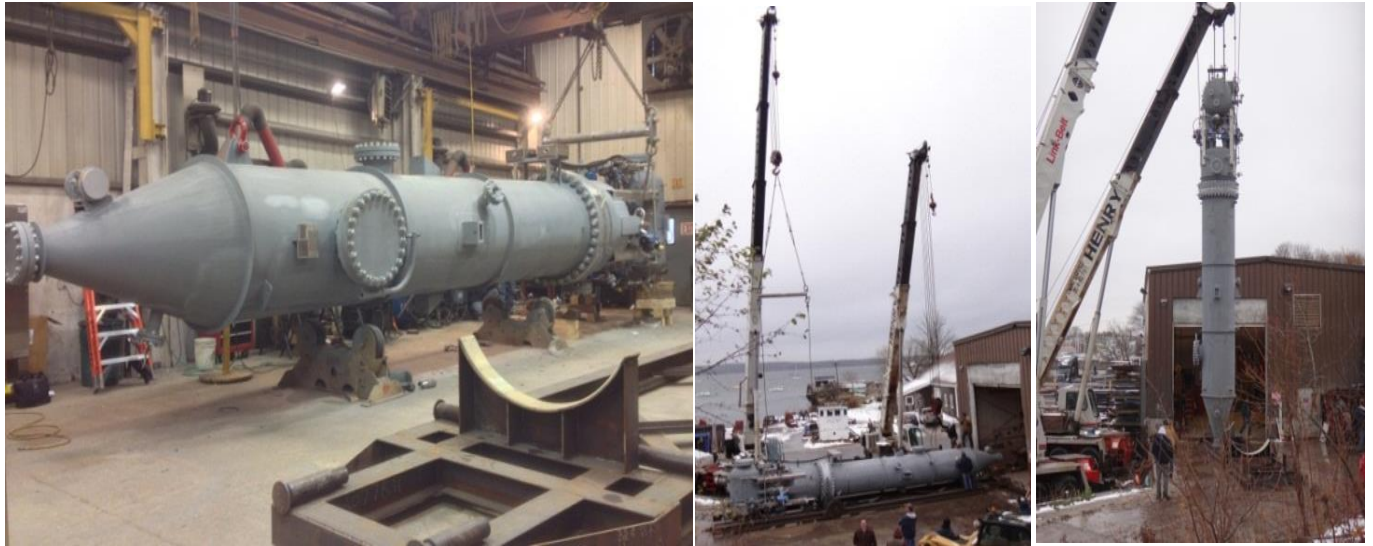
Figure No. 5.2: Mott GSV Filter Vessel: Assembled For Shipment & Lift
