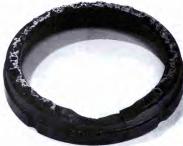
FIGURE 15. Example of pocked or cratered carbon washer. Typical of failures seen in model 4925 pumps with heavy (viscous) oil.
