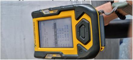
Performed random spot positive material identification test with satisfactory results on material type SS-304 and reviewed Equipromex QC PMI reports of SS components with positive results on MOC SS-304.
