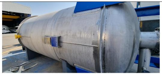
90 degrees view. Fabrication of water wash reactor W503W.2 is complete and ready for shipment. Final visual appearance of base metal and welding are satisfactory. Verified that MOC complies with the fabrication drawings with EQUIPROMEX PMI reports and MTR's.
