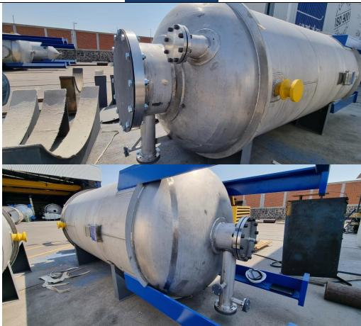
Top and bottom dished ends. Thickness after forming is over ½".
