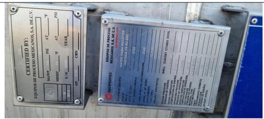
ASME nameplate, waring plates and data plate are properly attached.
