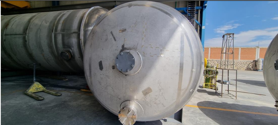
Top view. Verified top dished end thickness after forming is over 3/16".
