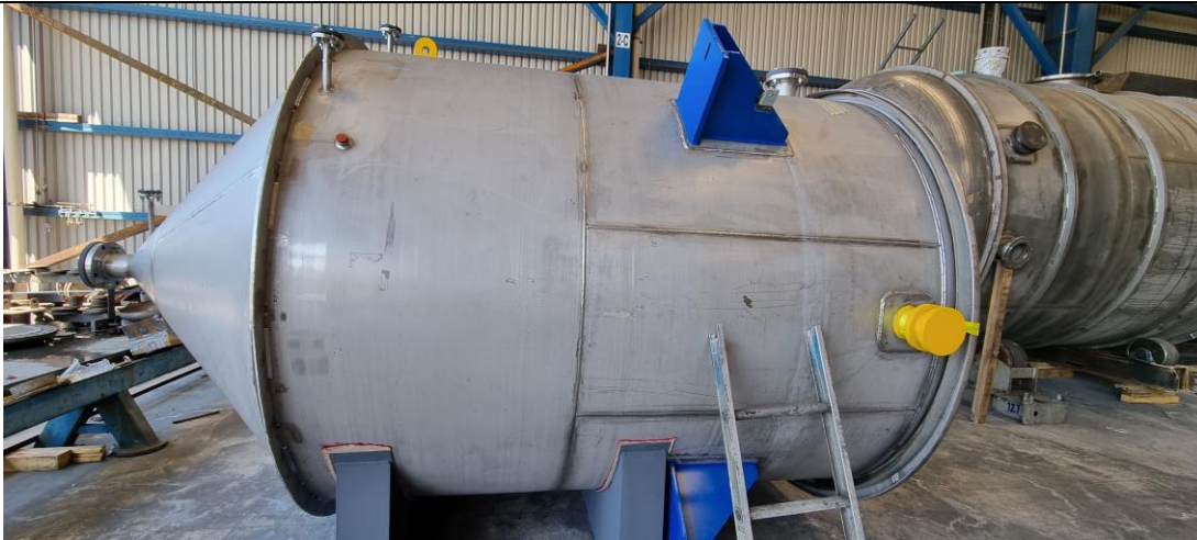
270 degrees view. External visual inspection satisfactory, base metal and welding final appearance ok.
