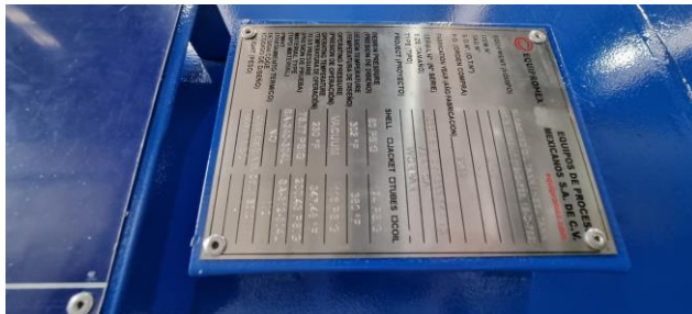
ASME plate and nameplate are properly attached. Both plates are with imperial units.
