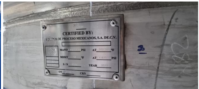
ASME plate and nameplate are properly attached. Both plates are with imperial units.
