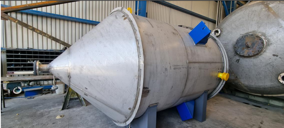
270 degrees view. External visual inspection satisfactory, base metal and welding final appearance satisfactory. Tank is ready for shipment.
