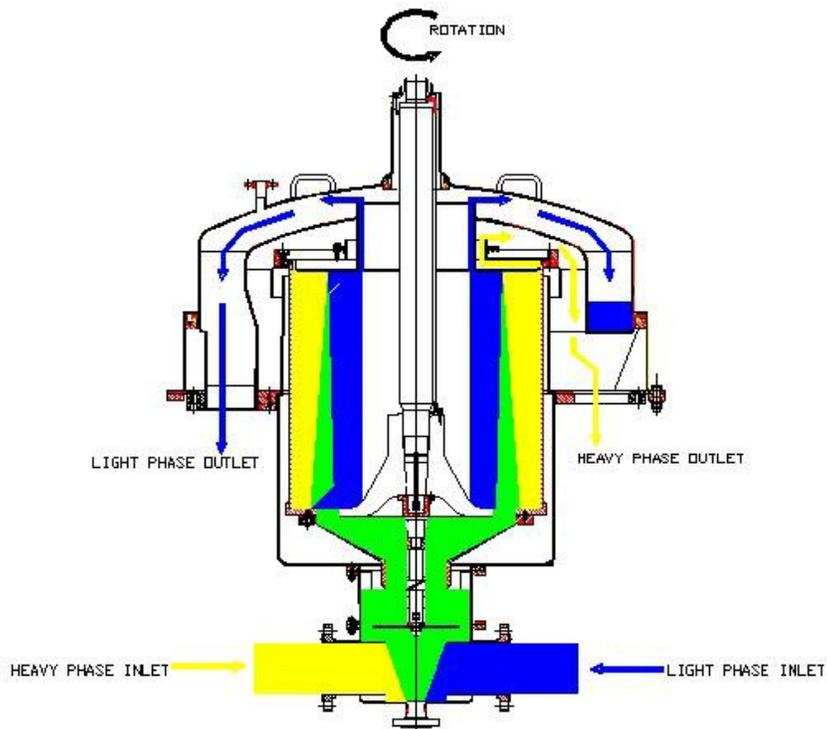
**Figure 2. Single stage Rousselet Robatel BXP extraction flow diagram.**
