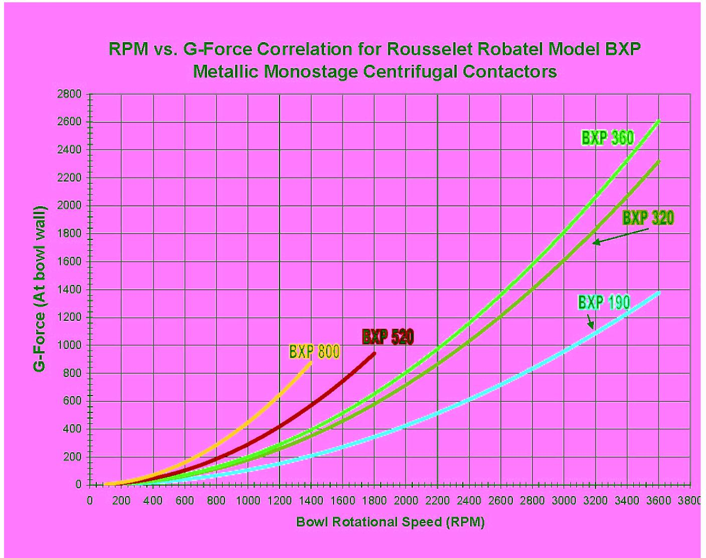
**Graph 3. G-force at bowl wall vs. rotational speed for Mono-stage BXP metallic extractors.**
