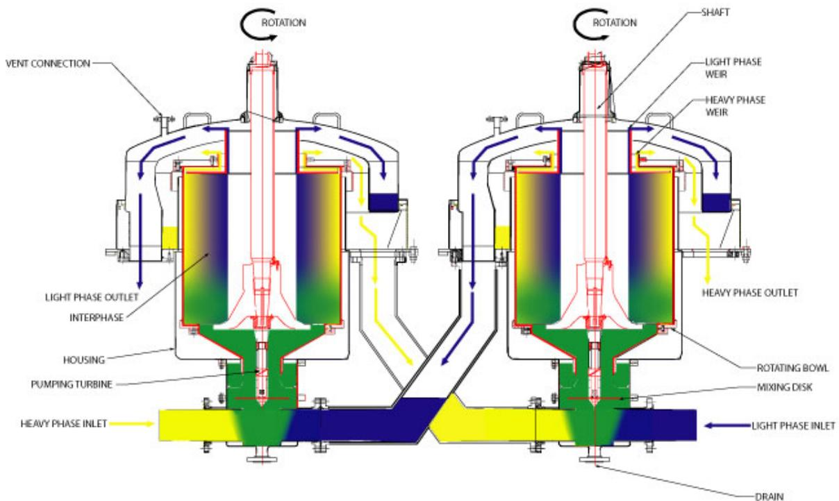
**Figure 3. Rousselet Robatel BXP 2 stage counter current extraction liquid flow diagram.**
