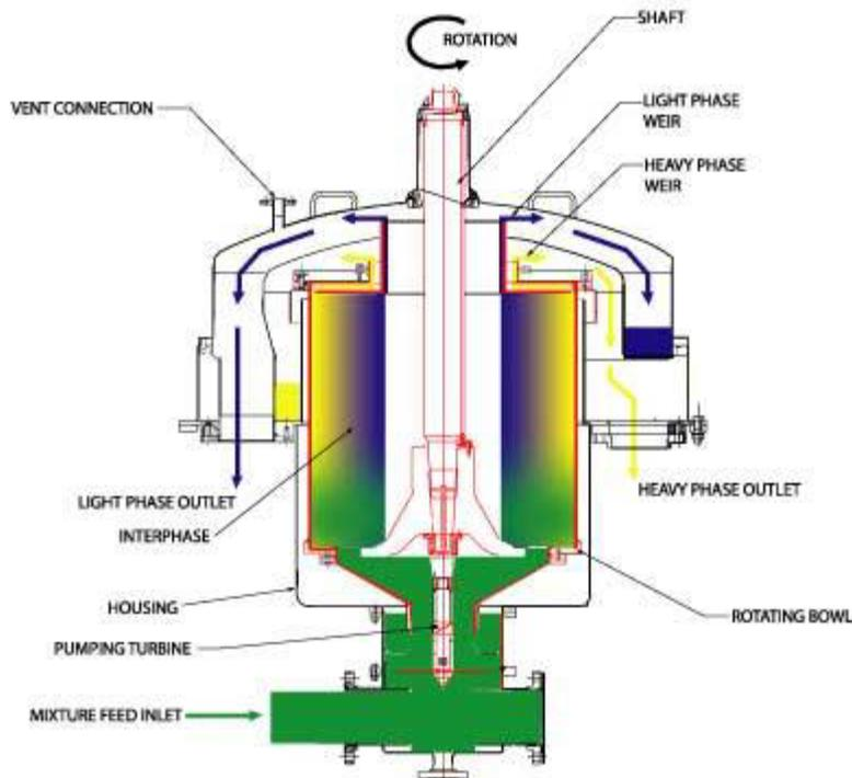
**Figure 1. Single stage Rousselet Robatel BXP centrifugal separator.**
