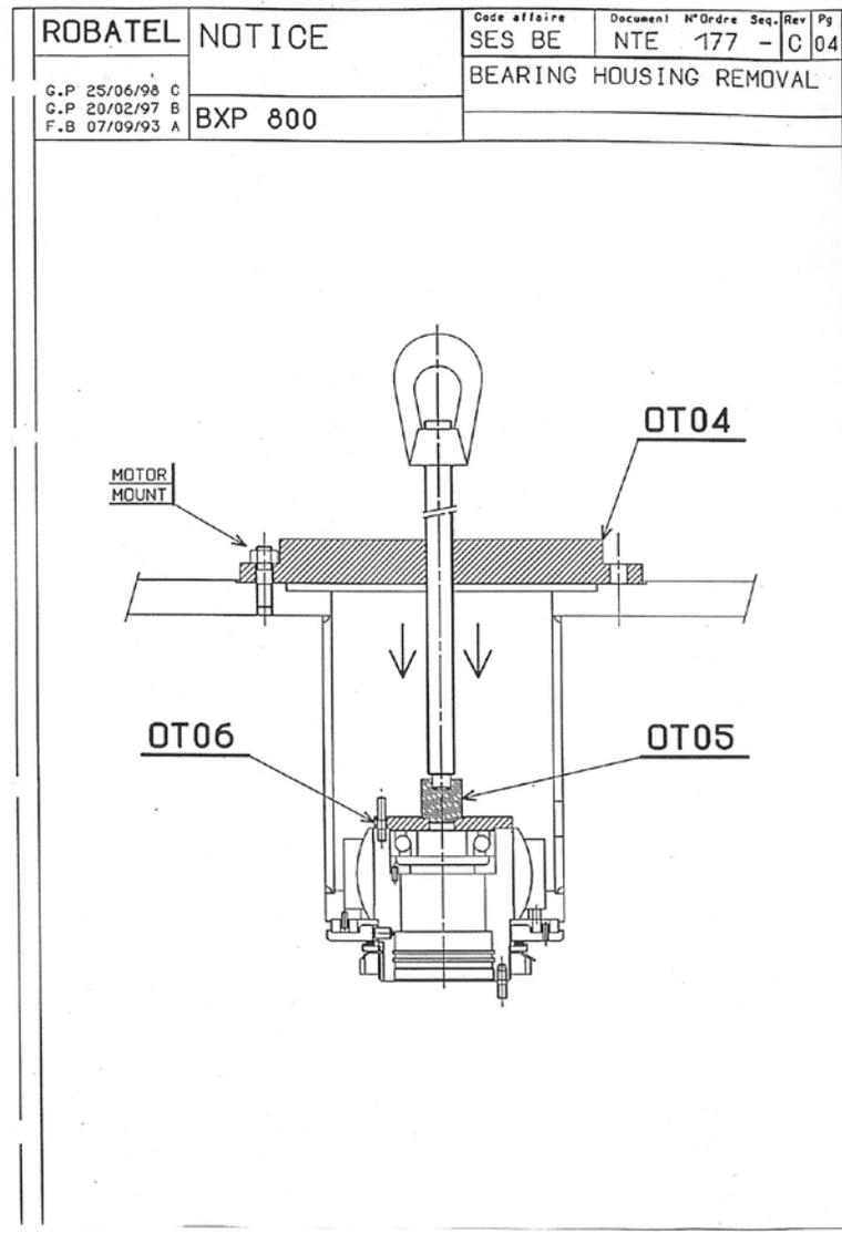
**Figure 11. Page 4 of the disassembly / reassembly sketches.**
