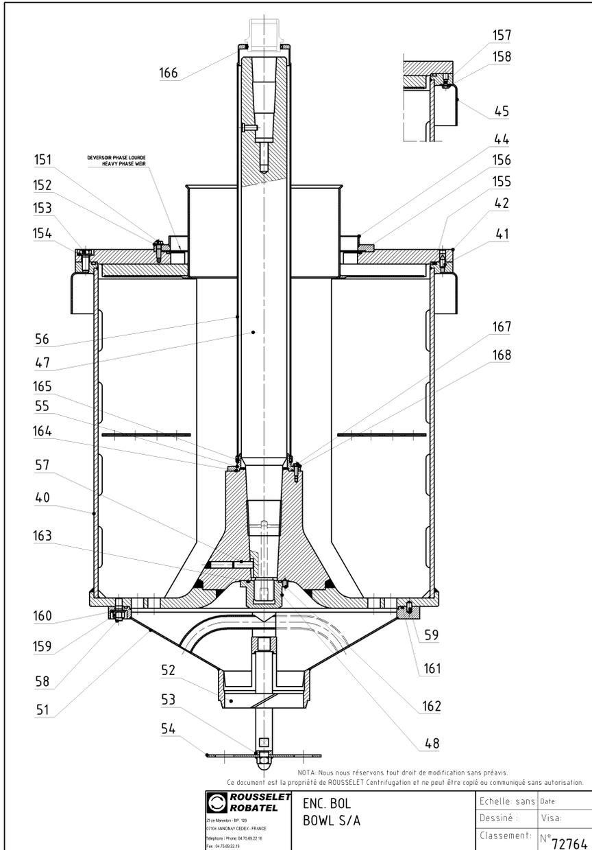
The bowl (ITEM NO. 40, DRAWING NO. 72764) has an internal diameter of **800 mm**, a useful volume of **320 liters**, and rotates at a speed of **1400 rpm** at **70 Hz**.
