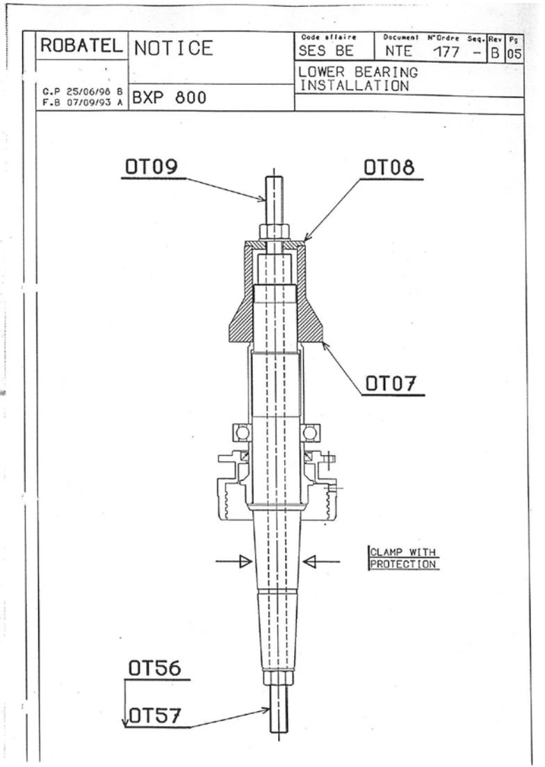
**Figure 12. Page 5 of the disassembly / reassembly sketches.**
