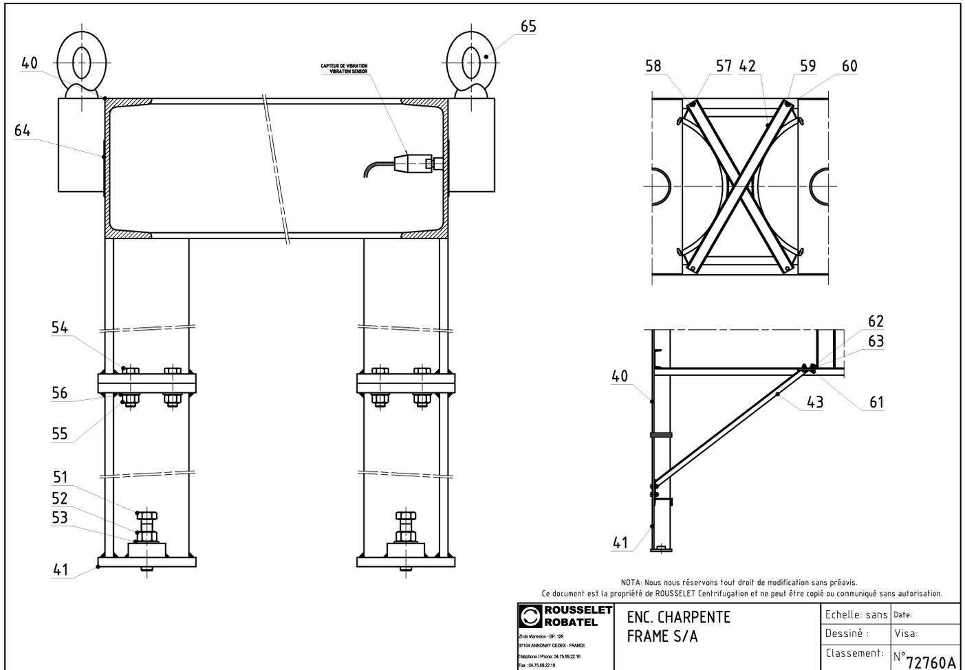
The support frame is equipped with legs and braces which are removed for shipment.
