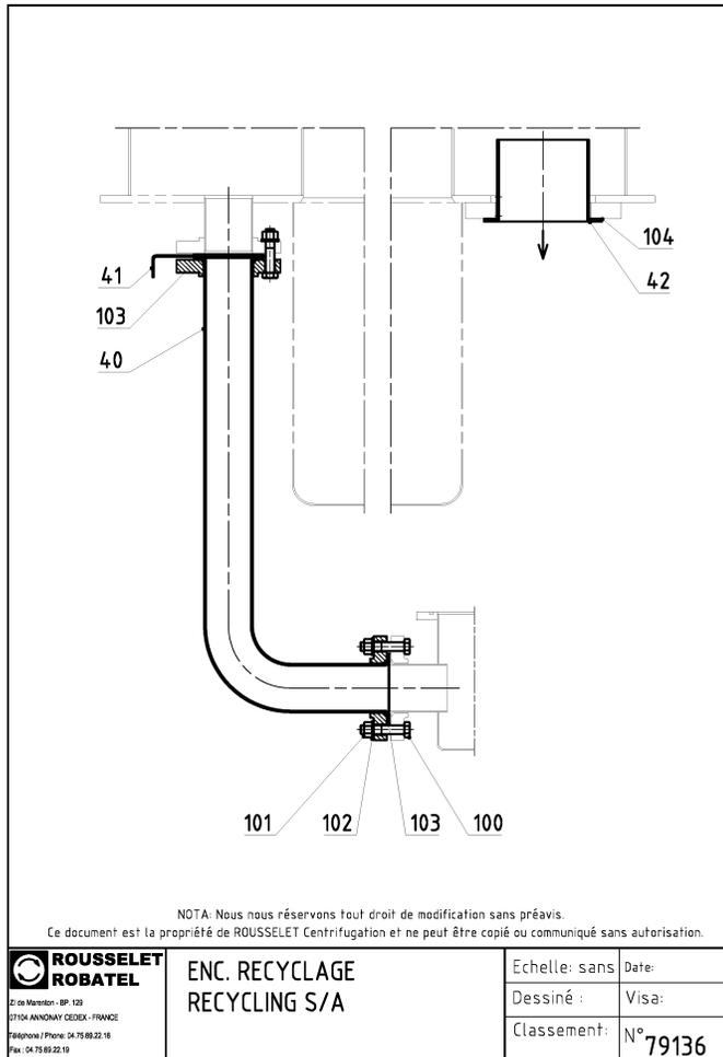
The casing of one stage is equipped with a recycling system for the heavy phase.
