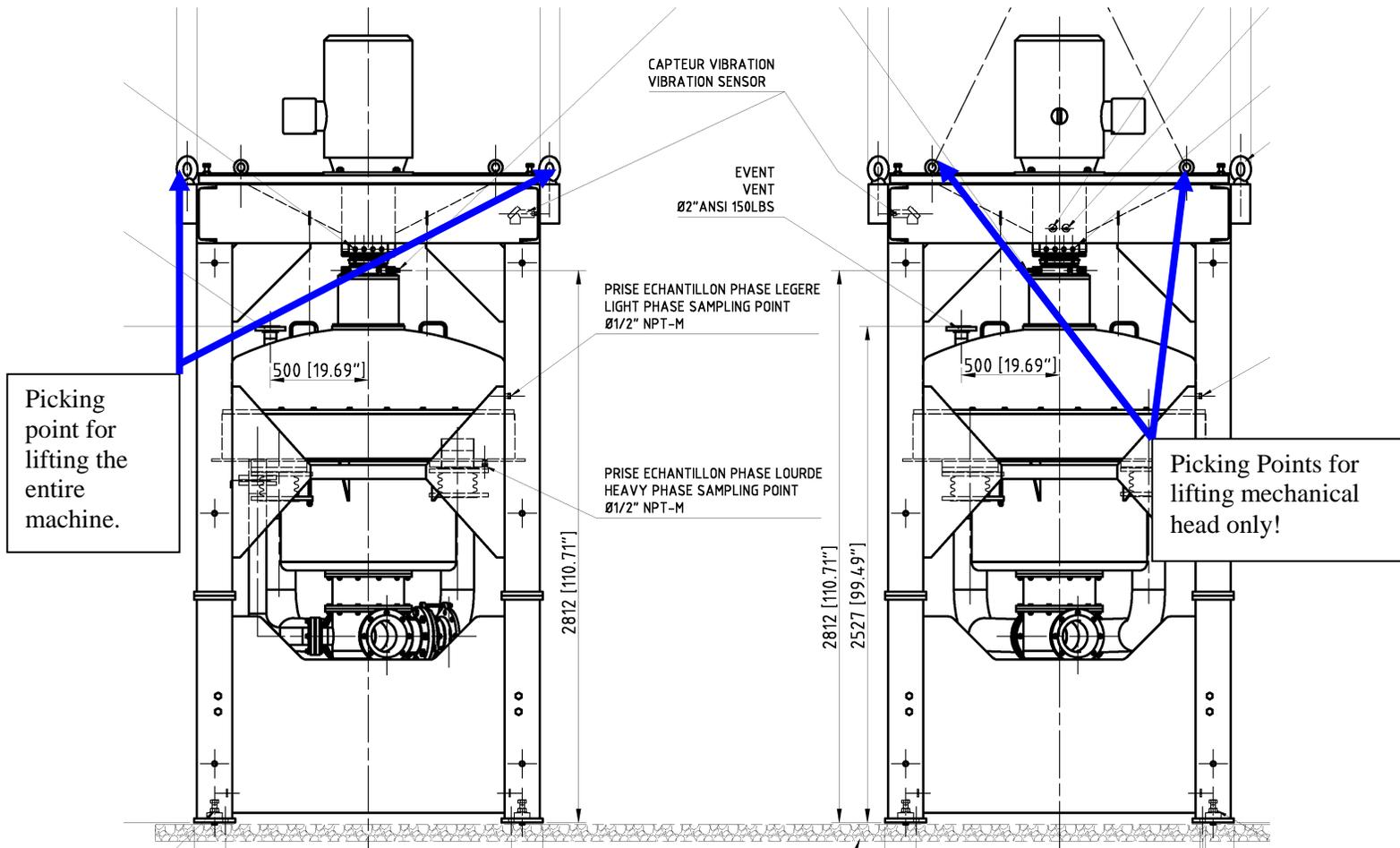
**Figure 4. Extractor lifting points.**
