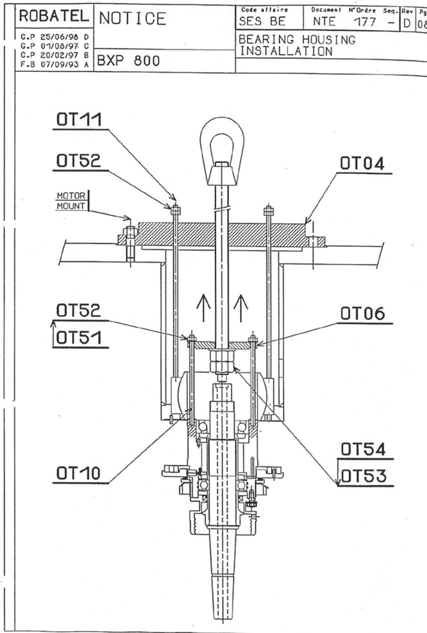
**Figure 15. Page 8 of the disassembly / reassembly sketches.**
