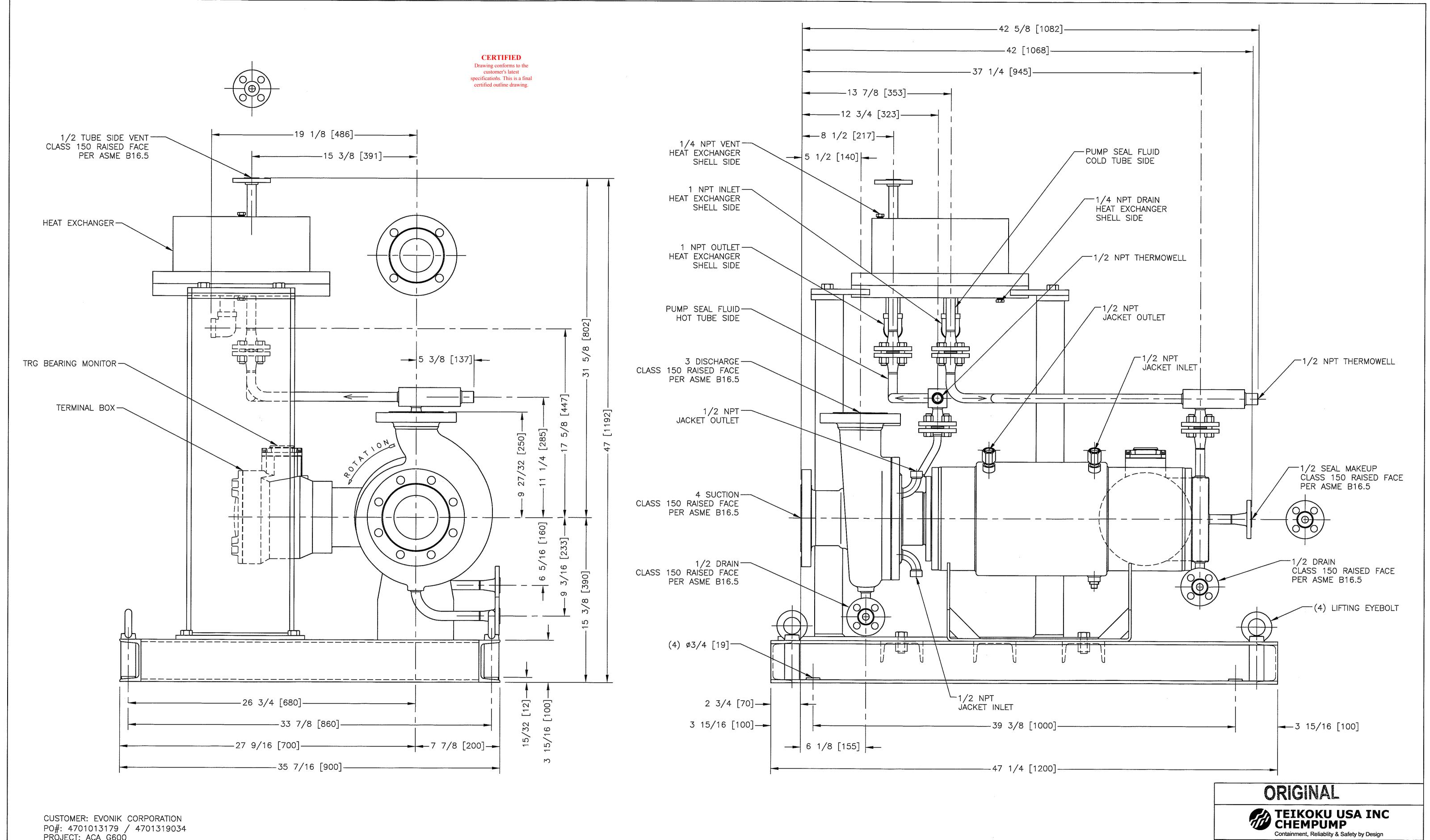
PRÖJECT: ACA G60Ó PROJECT#: 4142.00940 EVONIK'S PUMP#: P-1020/P-1020S REQUISITION#: CO078-010 WEIGHT: 1120 LBS. PUMP AND HEAT EXCHANGER WILL HAVE 2" OF CELLULAR GLASS INSULATION.
