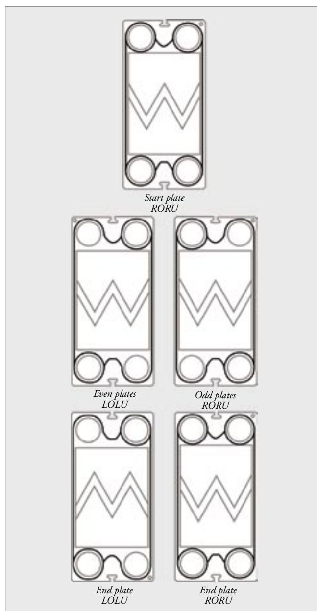
Figure 46 Gasket attaching orientation.
