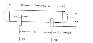
Weight on left saddle, op = 25568, test = 26042 lb Weight on right saddle, op = 24222, test = 24610 lb
