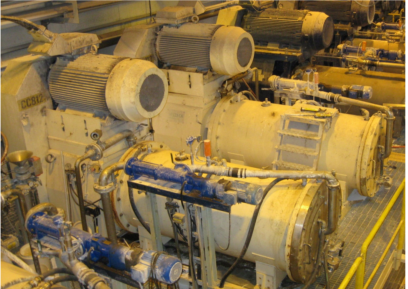
Fig 1. Horizontal Agitated Media Mill, LME 1000 K
