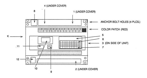
Figure 1-5. SLC 150 Programmable Controller.
