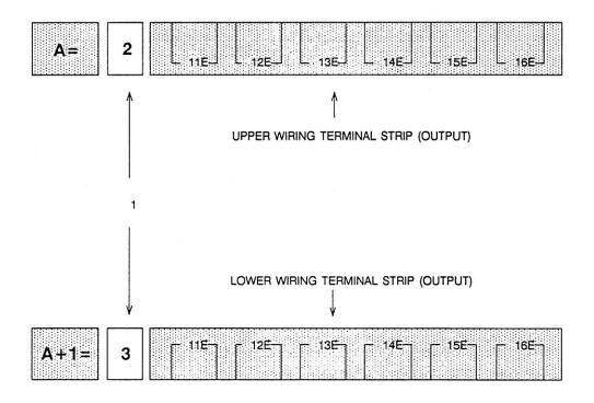
Figure 1-7. EU Address Block Numbering. (Item #7 in Fig. 1-6)
