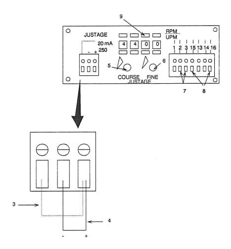
Figure 2-14. Speed Indicator (Adjustment).
