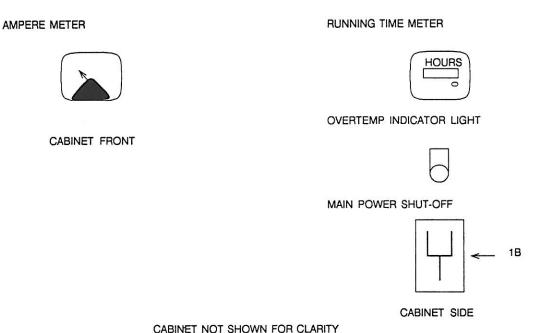
Figure 2-2. Starter Controls for MSD 90, 130, 170, 200, 250 Machines.
