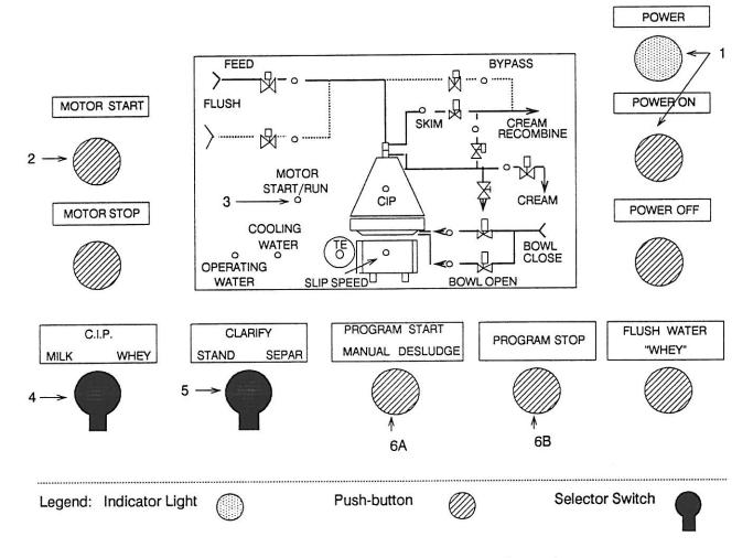
Figure 2-4. Control Cabinet, Separator Controls.
