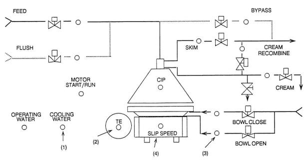
Figure 2-13. Illuminated Graphics Panel (Malfunction Indications).
