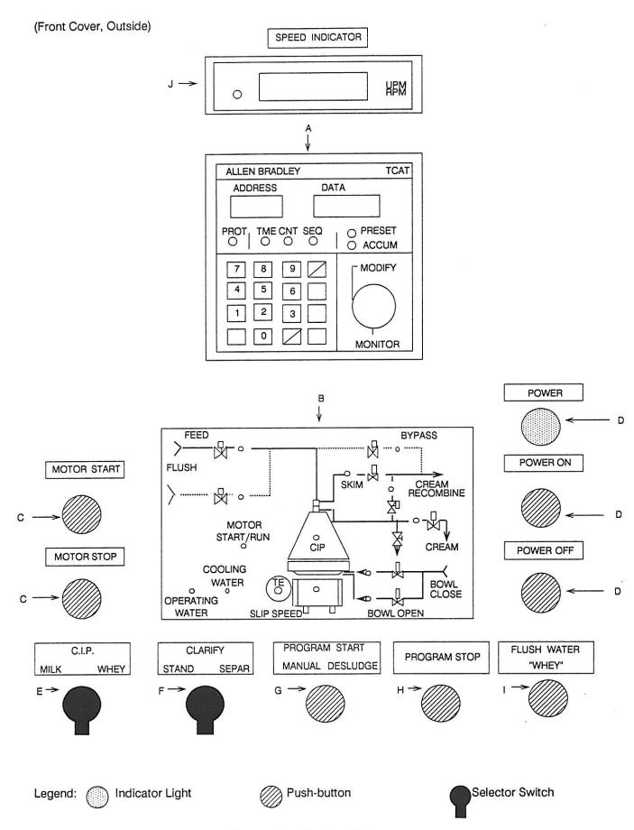
Figure 1-2. Control Cabinet. (Sheet 1 of 3)
