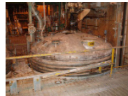
98579- 9300 Gallon 10' x 15'6" 15 Shell psi 304LSS Gaston County with Jacket and .75 hp agitator
