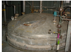
98579- 9300 Gallon 10' x 15'6" 15 Shell psi 304LSS Gaston County with Jacket and .75 hp agitator
