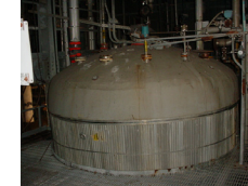
98579- 9300 Gallon 10' x 15'6" 15 Shell psi 304LSS Gaston County with Jacket and .75 hp agitator
